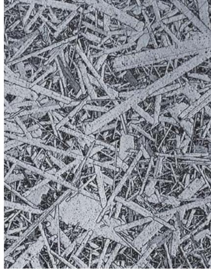
Grain size 10 – 1,500  $\mu\text{m}$ , density > 3.10  $\text{g/cm}^3$
