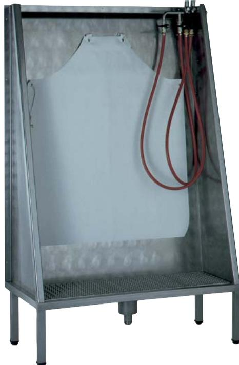
Made of stainless steel 1.4301. The washing facility features two side guards and a rear guard with hooks to hang up the aprons. The water supply of the brush is controlled by a globe valve and the centre drain is equipped with a dirt sieve. If you want to clean your boots, place them on the removable grid covering the basin and use the boot brush to clean off dirt and waste material.
