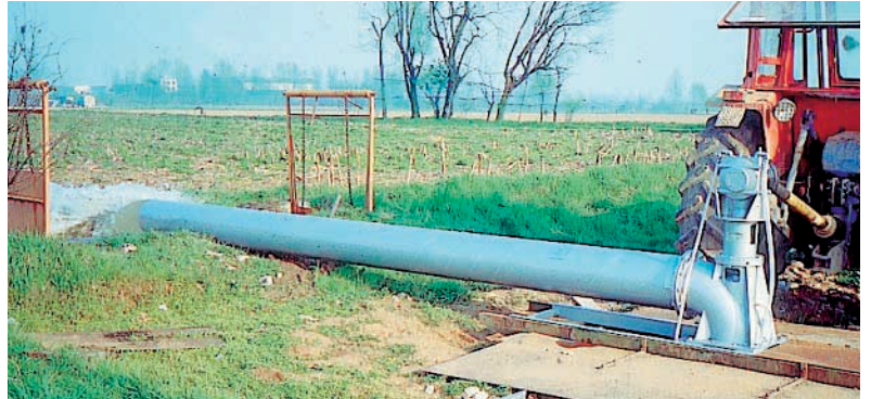
Driving the pump off the mortising-shaft of your tractor
