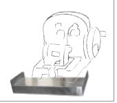
Simply place tray under Microtome -For safety's sake, remove knife from microtome before inserting tray.
