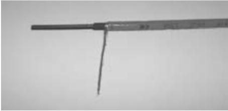
2. The screen is released and twisted. Following this, remove the outmost 80 mm of the primary insulation. Use knife.
