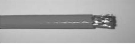
1. Remove 15 mm of the outer sheath. Remove the screen braid from the 15 mm stripped cable, too. Be careful not to damage the primary insulation.
