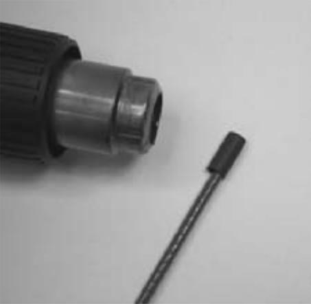
2. Crimp tube 6/2, L = 20 mm is pulled in over the end of the cable to the edge of the removed outer sheath. 5 mm of the crimp tube must still be free of the cable.
