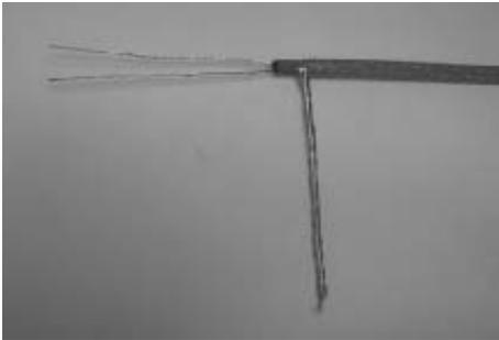
3. The core material is removed from the conductors, also from the outmost 80 mm. Be careful no to damage the conductors.
