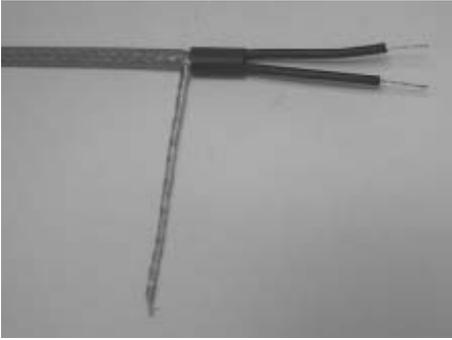
6. Crimp tube 9/3, L=20 mm is pulled in over the two conductors, all the way to the twisted screen in order to cover approx. 10 mm of the primary insulation and approx. 10 mm of the conductors.
