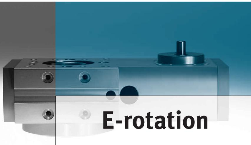
Weights of up to 15 kg can be rotated dynamically and flexibly with the freely positionable, electric rotary drive module ERMB. The ERMB can naturally be systematically incorporated in a mechatronic multi-axis modular system: as a phi axis with any rotation angle  $>360^\circ$  or “stand alone” as a small NC controlled rotary table.
