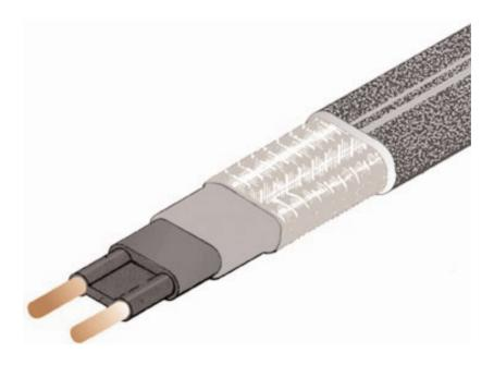
The Devi Pipeguard is a self-limiting parallel heating cable. The power output of the conductive core material increases or decreases in response to ambient temperature changes.
