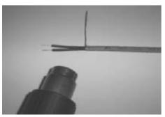
5. The crimp tube is crimped down from the core material towards the cable end.
