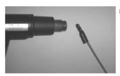
The end sealing is crimped down from the sealed end and in over the cable.
