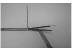
The crimp tube is crimped down and immediately after this the outmost 10 mm are squeezed together on the middle with flat pliers.
