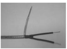
8. Yellow/Green, L=50 mm tube is pulled in over the twisted screen.
