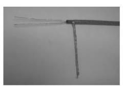
The core material is removed from the conductors, also from the outmost 80 mm.
