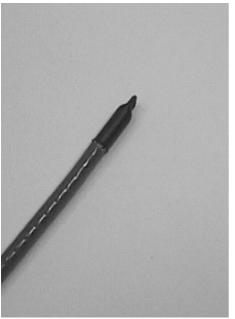
The crimp tube is crimped down, whereafter the outer 5 mm is squeesed with a pliers.
