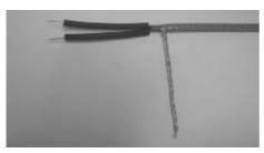
4. Crimp tube 4/1, L=70 mm is pulled on to the two stripped wires.
