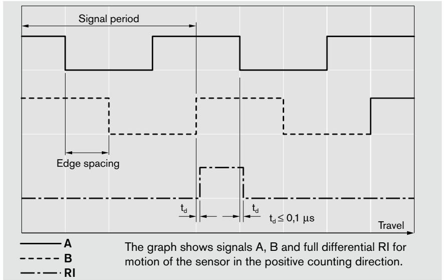
Motion direction for positive counting of sensor signals
