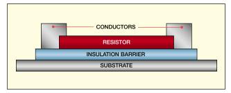
Thick Film Heater Construction
