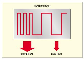
Varying Heat by Varying Circuit Density
