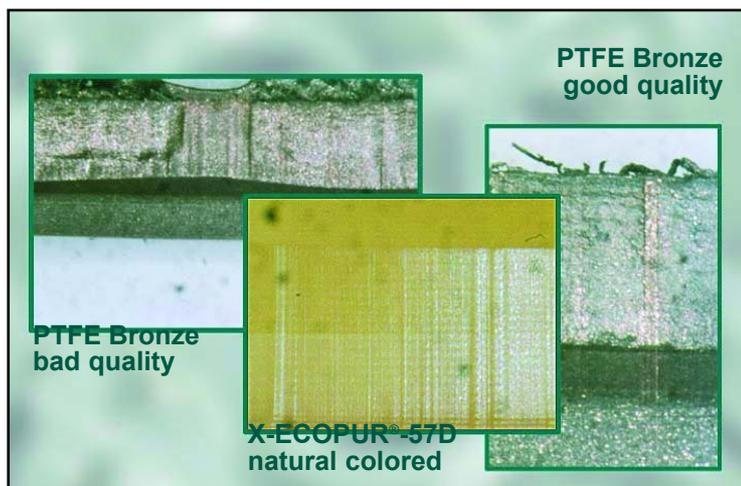
Fig. 15: Microscopic investigations of the sliding surface of composite seals
