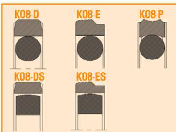
Fig. 1: Examples of co-axial and in-line composite seals for piston sealing
