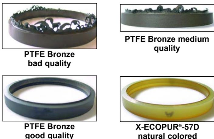
Fig. 14: Gap extrusion and wear of composite seals
