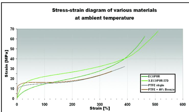
Fig. 8: Stress-strain graphs of sealing materials
