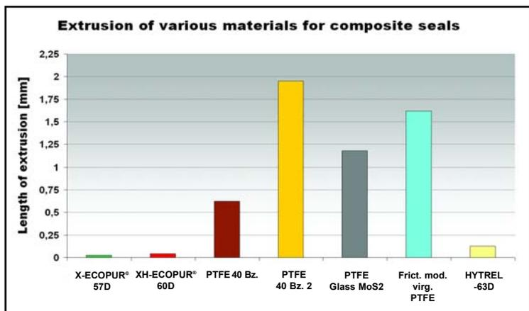
Fig. 13: Gap extrusion of composite seals
