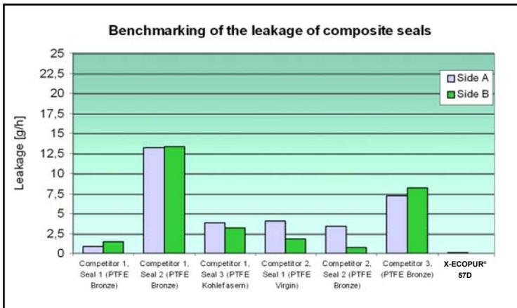
Fig. 17: Leakage characteristics of commercially available composite seals compared to X-ECOPUR®-57D
