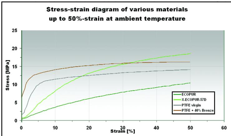
Fig. 6: Stress-strain graphs of various sealing materials
