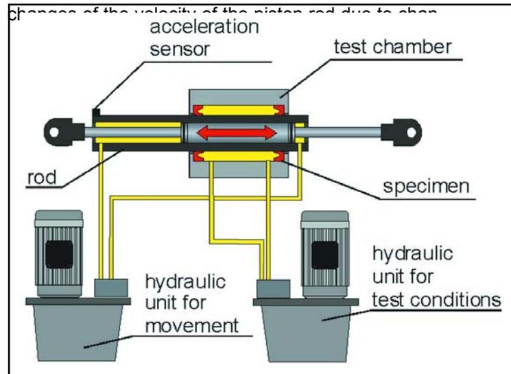
Fig. 5: Scheme of the test rig for stick-slip investigations
