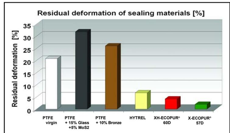
Fig. 10: Tensile set of various sealing materials
