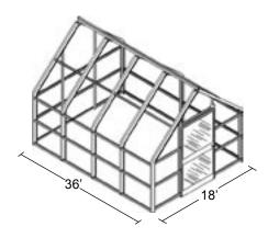
This greenhouse is engineered to meet 70 mph wind and 10 pound live load per the UBC Building Code. Higher load ratings and stamped engineered plans are available at extra cost. All galvanized steel frame insures maximum strength and life. Lexan twin-wall polycarbonate covering is UV resistant with a 10 year discoloration warranty.
