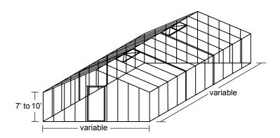
Cross Country Greenhouses are engineered to meet 80 mph wind and 30 pound live load per the UBC Building Code. These structures are designed to meet the building code requirements in most states. If you have questions or special needs, call IGC customer service for pricing on any custom requirements.
