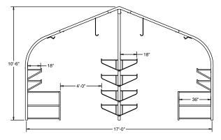
The Shelfmate Teaching Package is NOT a load-rated structure, but features a sturdy, galvanized steel frame that easily snaps together. The structure can be secured with ground stakes on turf or weighted water tubes. Horticultural classes can set up the Shelfmate greenhouse as needed and disassemble and store it when school's out. The built-in shelves make it a convenient all-in-one package. Call IGC customer service if you have questions or for pricing on any custom requirements.
