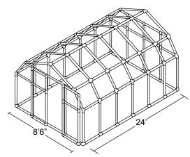
Features UV protected PVC profiles and 4mm twin wall polycarbonate panels with a 10 year discoloration warranty. Although made of PVC, the Rion greenhouse is roof tested to hold an incredible 1,100 pounds of snow! Despite this testing, please note that these greenhouses are NOT load rated structures.
