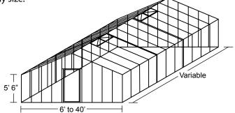
IGC glass greenhouses are also available with a curved eave and can be made to build on a knee-wall or glass to ground. Available in bronze, green or white. All IGC Glass Greenhouses are engineered to meet 70 mph wind and 10 pound live load per the UBC Building Code. For an additional expense, your structure can be designed to meet any building code requirements for live and/or wind load. Call IGC customer service for pricing on any custom requirements.
