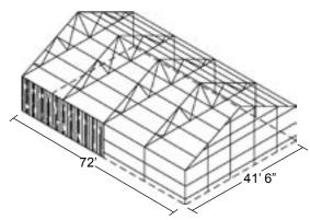
This greenhouse is engineered to meet 70 mph wind and 10 pound live load per the UBC Building Code. Higher load ratings and stamped engineered plans are available at extra cost. All galvanized steel frame insures maximum strength and life. Lexan corrugated polycarbonate covering is UV resistant with a 10 year discoloration warranty.
