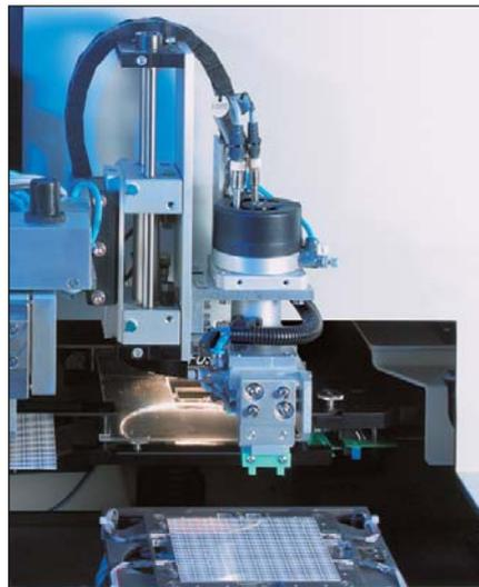
Fig. 12: Laser trimming of platinum-chip temperature sensors
