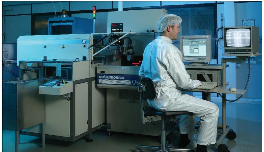
Fig. 6: Producing temperature sensors under clean-room conditions
