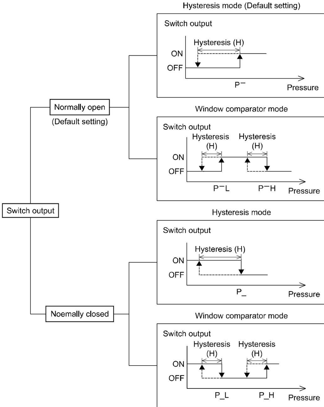
If the point where the switch output is changed comes outside of set pressure range due to the change of set pressure, hysteresis(H) is automatically compensated.
