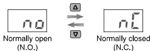
3. Keep pressing the
