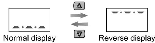
3. Keep pressing the
