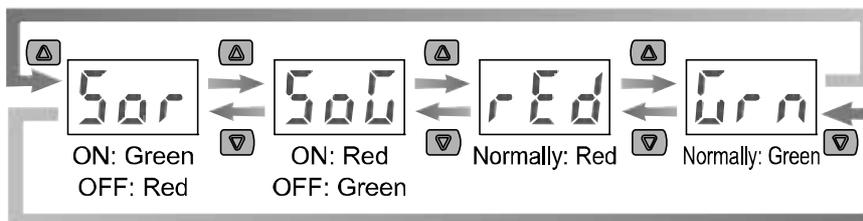
3. Keep pressing the
