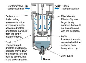
The compressed air introduced from the inlet is given circling movements by the deflector. The resulting cyclone effects forcibly push comparatively large free droplets and foreign particles toward the inner walls of the bowl, causing them to move down the wall surfaces and accumulate in the bowl's bottom.
