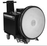
Using the handle, the head can tip 90° from the operating to the pad change position.
