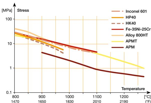
Figure 1 Creep rupture strength – 10 000 h.
