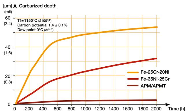
Figure 5 Carburization resistance.
