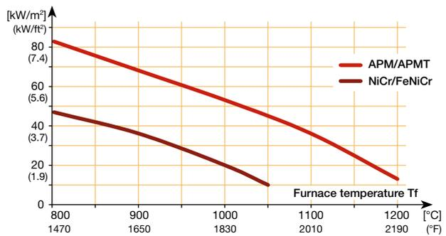
Figure 7 Power output SER-burner systems.
