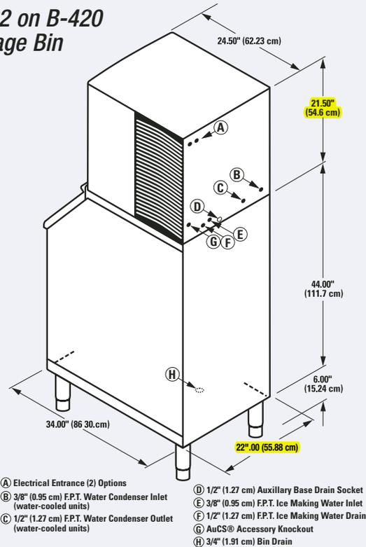
**Installation Note** - Minimum installation clearance—Top: 12" (30.48 cm); Sides: 8" (20.32 cm); Back: 5" (12.7 cm).
