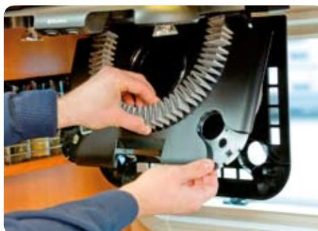
Exchangeable activated carbon filter
