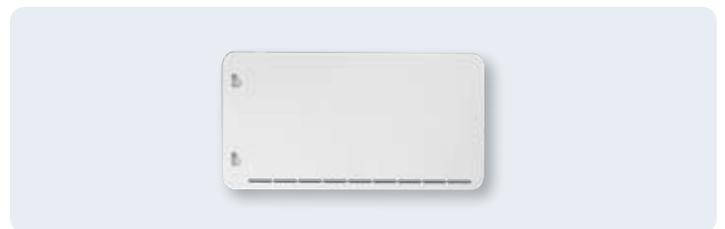
**Winter set for LS 300 for two-door models:** The polyurethane foam ventilation grill gives this refrigerator particularly high insulation values. Even at ambient temperatures as low as  $-30^{\circ}\text{C}$  the winter set ensures maximum performance from the absorption unit when running on gas or electricity. At temperatures above  $5^{\circ}\text{C}$  we recommend using a standard cover.
