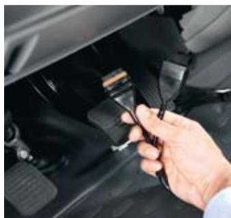
Connection to the accelerator via T-plug
