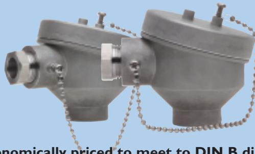
This housing is available in SS 316, and is economically priced to meet to DIN B dimensions and requirements. It can accommodate a medium sized temperature transmitter or terminal block, 50 mm in diameter. The PGI6 version only comes with a cable gland. The processide dimensions are identical to the DIN B head, so they can replace them in full. Weight for the SS 316 version, 360 gram.
