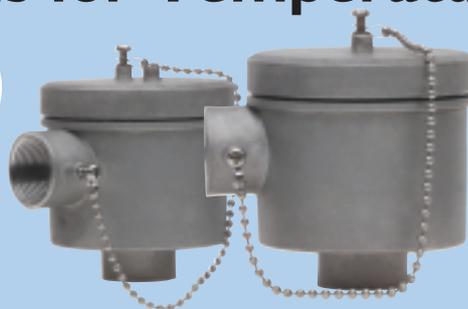
This housing is available in SS 316, and is designed specially for large temperature transmitters. The housing will accommodate a transmitter 65 mm (2.5") in diameter and approximately 45 mm (1.8") in height. Meets the requirements of IP65 NEMA 4. Weight for the SS 316 version, 560 gram.
