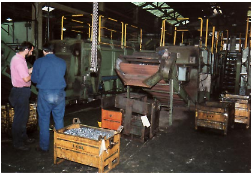
There are four electrically heated link-belt furnaces at T.T.T. for hardening of nuts and bolts. Each furnace has 12 Tubothal elements in the first zone rated at 5 kW in vertical position.
