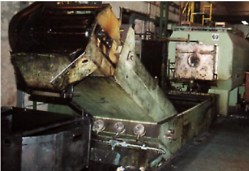
One rotating furnace with 24 Tubothal x 3.6 kW in the two first zones. The APM tubes are of 87 mm outer diameter.
