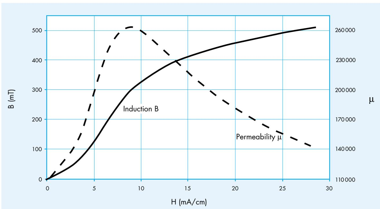
Figure 2 - Typical DC permeability and induction field-strength curves of Magnifer 8105 measured using stamped rings of thickness 0.55 mm annealed for 3h at 1050 °C.
