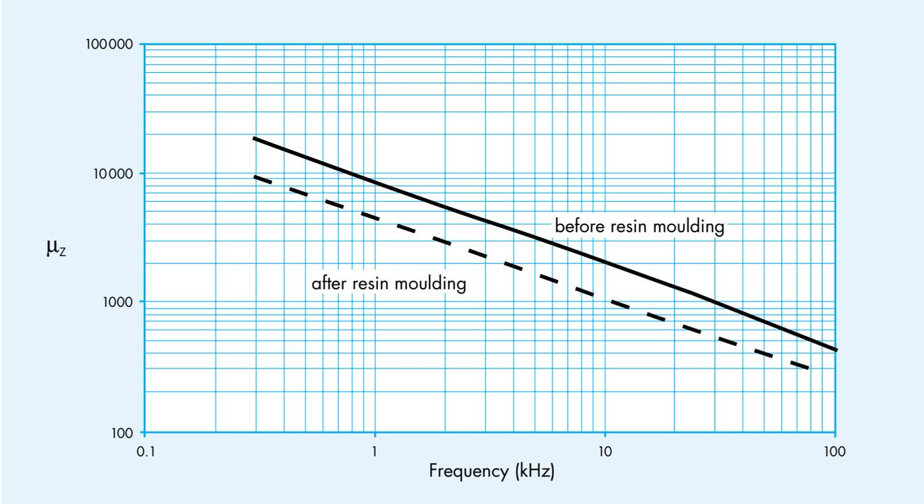
Figure 7 - Typical curves of the impedance permeability  $\mu_z$  of Magnifer 8105 in relation to frequency before and after resin moulding measured using stamped rings of thickness 0.55 mm annealed for 3h at 1050 °C.
