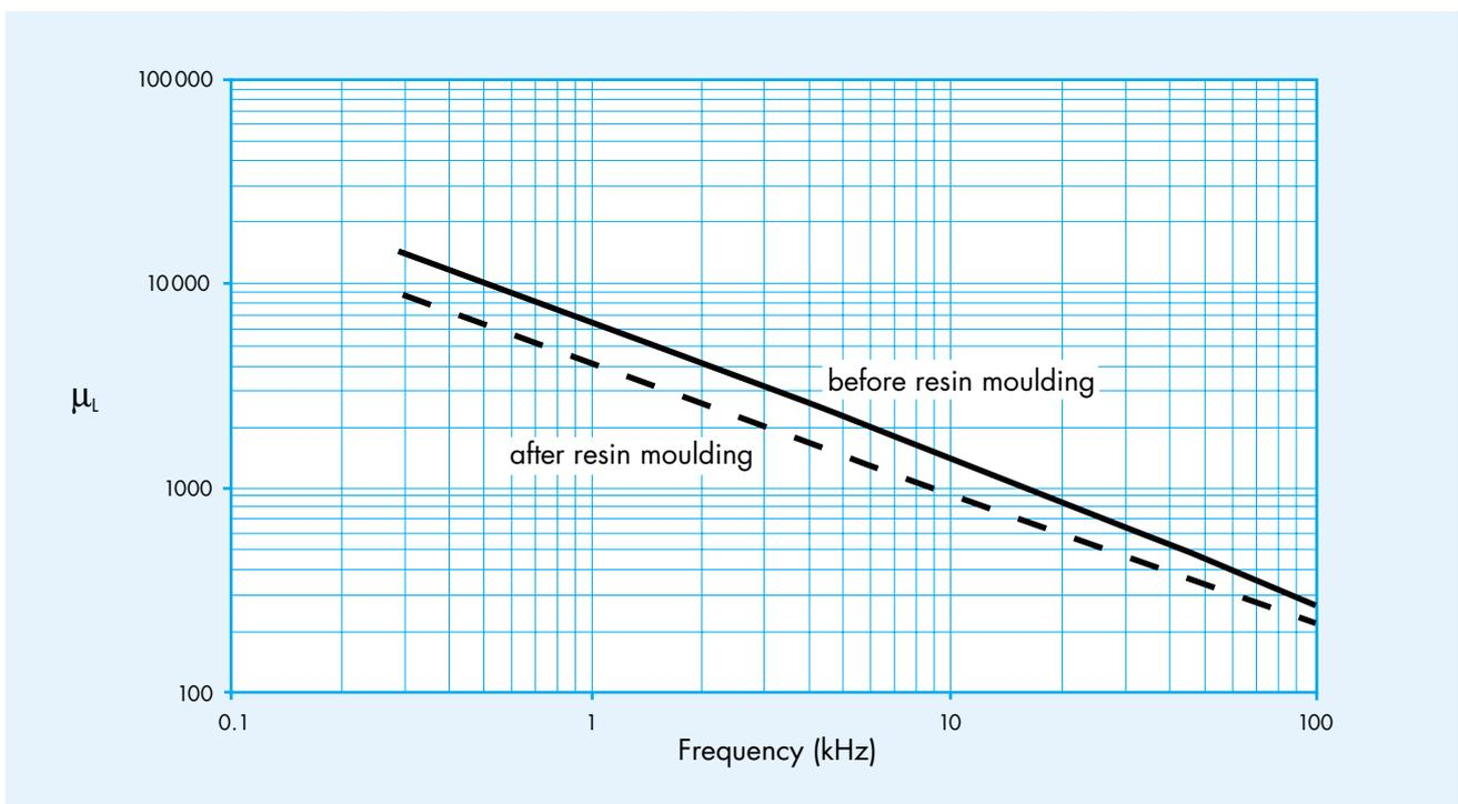
Figure 10 - Typical curves of the inductance permeability  $\mu_L$  of Magnifer 8105 So in relation to frequency before and after resin moulding measured using stamped rings of thickness 0.55 mm annealed for 3h at 1050 °C.
