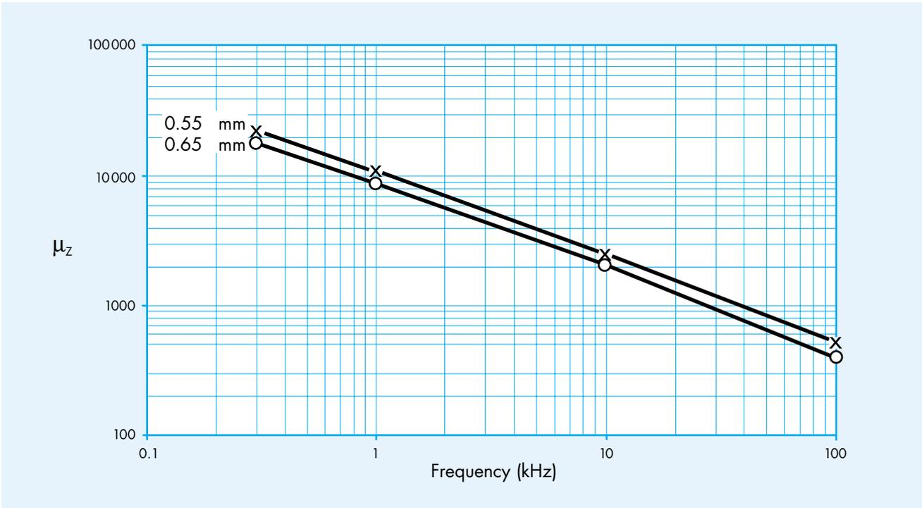
Figure 4 - Typical curves of the impedance permeability  $\mu_z$  of Magnifer 8105 So in relation to frequency and thickness.
