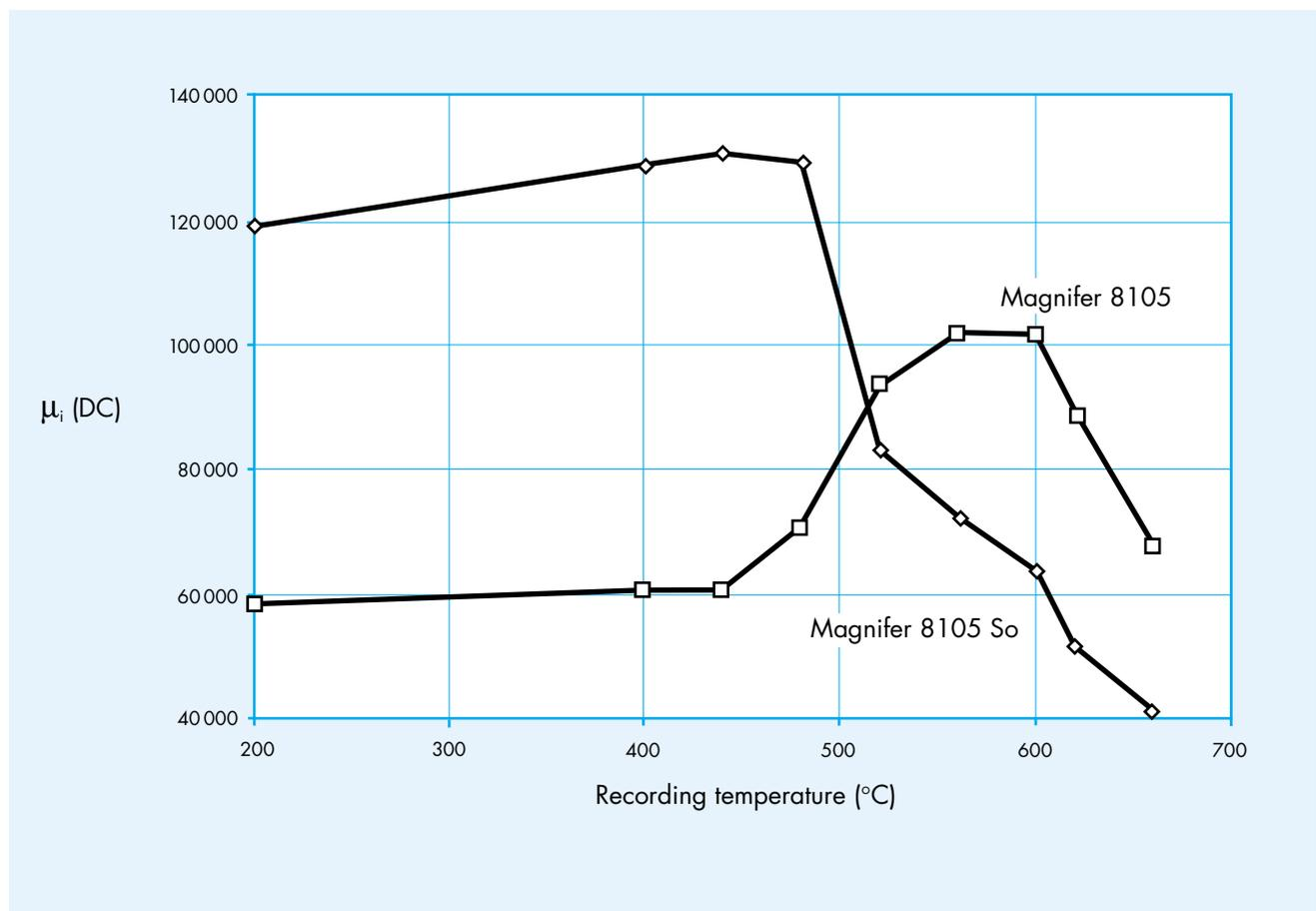
Figure 11 - Explanation of the different behaviour of Magnifer 8105 and Magnifer 8105 So depending on the temperature at which rapid cooling starts.
