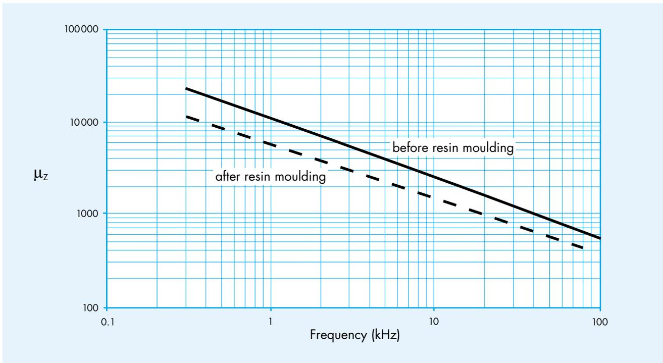
Figure 9 - Typical curves of the impedance permeability  $\mu_z$  of Magnifer 8105 So in relation to frequency before and after resin moulding measured using stamped rings of thickness 0.55 mm annealed for 3h at 1050 °C.
