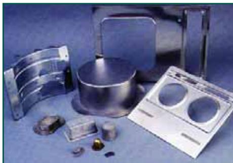
typical products of a high pressure hydraulic press
