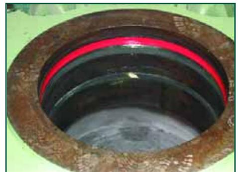
housing with installed H-ECOPUR® seal
