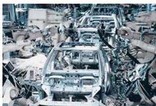
Hard-to-reach areas, for example, on welding lines in the automobile industry, which are secured by fences and where no access is possible.
