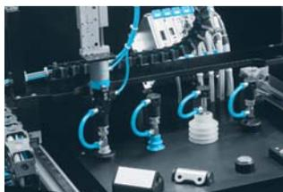
Different workpieces are processed on the same equipment using different pressures. This can be programmed with the LRE.
