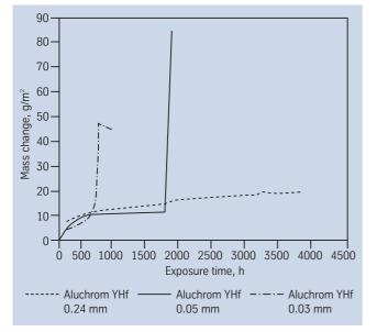
Fig. 1 – High temperature oxidation resistance of Aluchrom YHf strip in various thicknesses at 1100  $^{\circ}$ C (2012  $^{\circ}$ F) using 100 h cycles.
