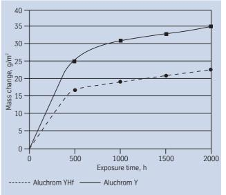
Fig. 2 – Comparison of high temperature oxidation resistance of Aluchrom Y with Aluchrom YHf at 1200 °C (2192 °F) using 100 h cycles.
