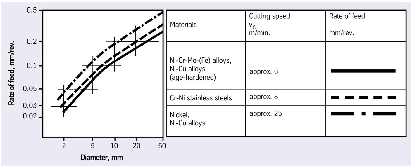
Fig. 5 – Guide values for cutting speeds and rates of feed in relation to tool diameter for drilling with HSS tools
