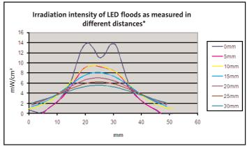
\* measured with Hönle LED area sensor for UV Meter
