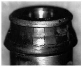
Photo 2 Cracking of check valve seal
