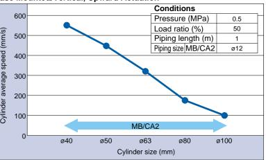
For details about the respective condition, make use of the SMC's Model Selection Program for air cylinder driving system for your reference.
