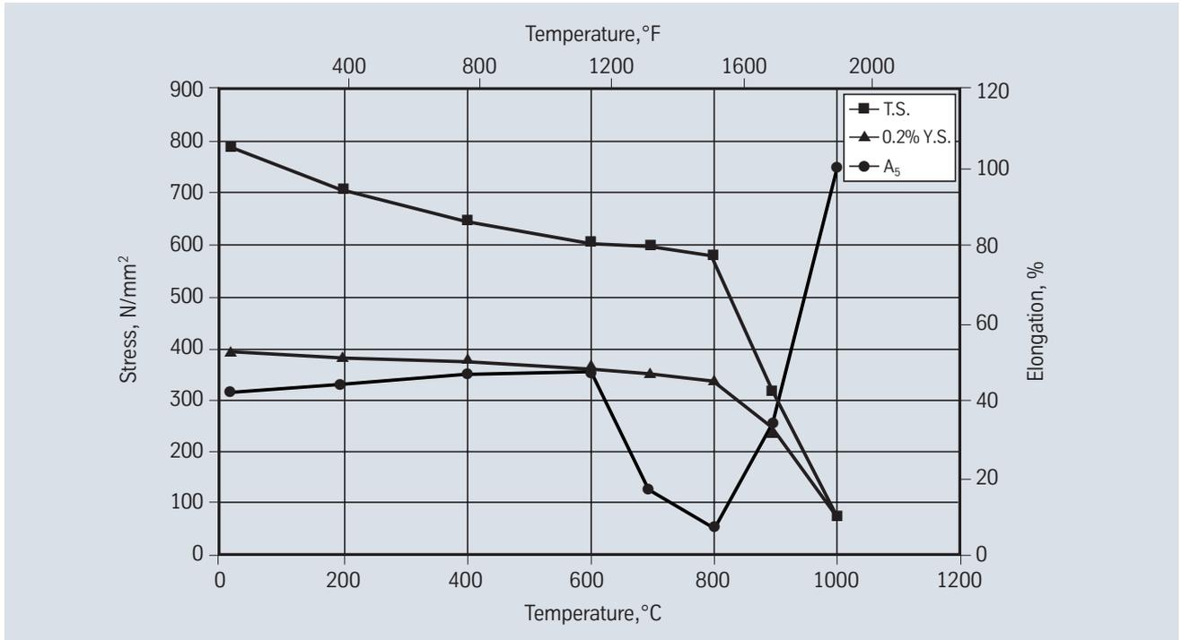
Fig. 1 – Typical short-time properties of solution-treated Nicrofer 7016 TiAl rod and bar products at room and elevated temperatures.
