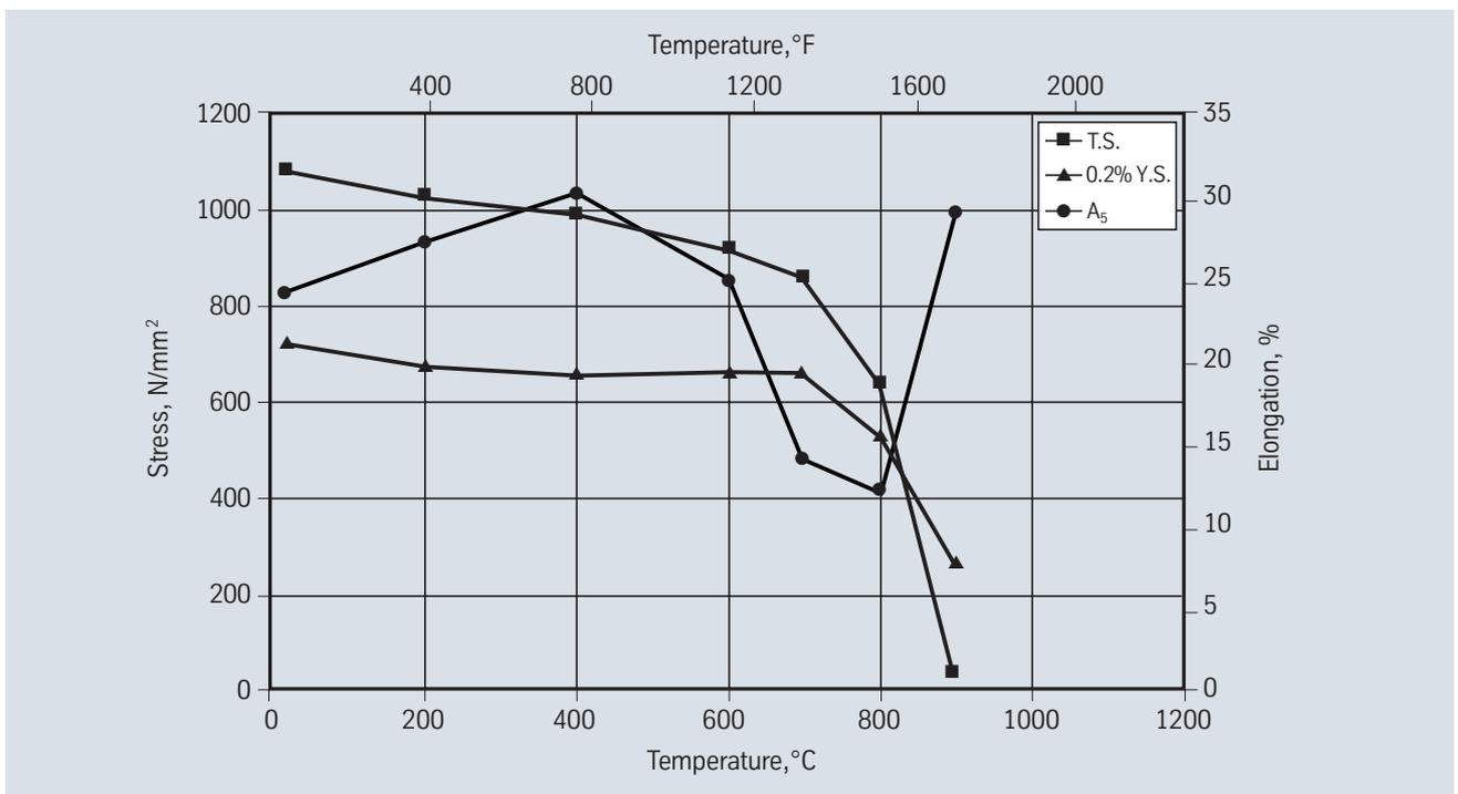
Fig. 2 – Typical short-time properties of solution-treated and age-hardened Nicrofer 7016 TiAl rod and bar products at room and elevated temperatures.
