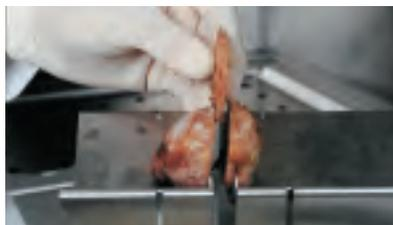
3. Raise the upper jaws and remove your 2 mm section from between the saw blades. The entire unit can be disassembled without tools for easy cleaning or disinfection.
