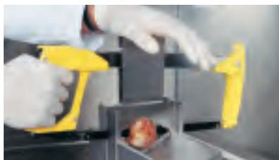
2. Insert the saw into the space between the upper jaws. The bone is immobilized by placing downward pressure on the upper jaws. Now simply use the saw to cut your section accurately.
