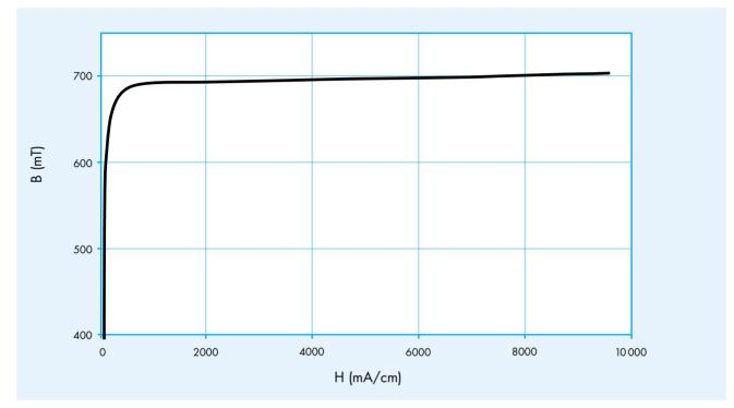
Figure 1 - Typical DC induction/field-strength curve of Magnifer 8105 measured using stamped rings of thickness 0.55 mm annealed for 3h at 1050 °C.
