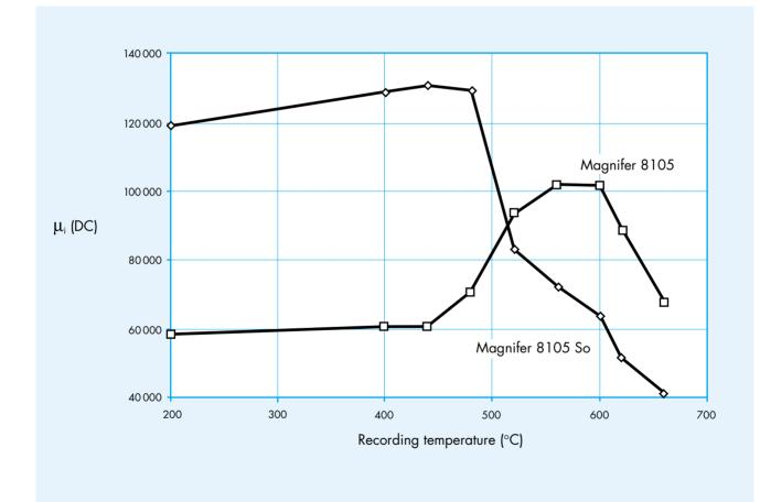
Figure 11 - Explanation of the different behaviour of Magnifer 8105 and Magnifer 8105 So depending on the temperature at which rapid cooling starts.
