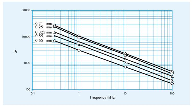
Figure 5 - Typical curves of the inductance permeability  $\mu_l$  of Magnifer 8105 in relation to frequency and thickness.
