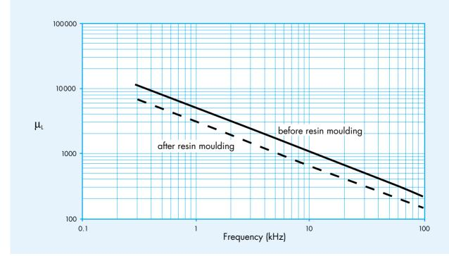
Figure 8 - Typical curves of the inductance permeability μ<sub>L</sub> of Magnifer 8105 in relation to frequency before and after resin moulding measured using stamped rings of thickness 0.55 mm annealed for 3h at 1050 °C.
