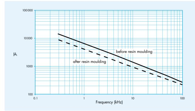
Figure 10 - Typical curves of the inductance permeability µ<sub>L</sub> of Magnifer 8105 So in relation to frequency before and after resin moulding measured using stamped rings of thickness 0.55 mm annealed for 3h at 1050 °C.
