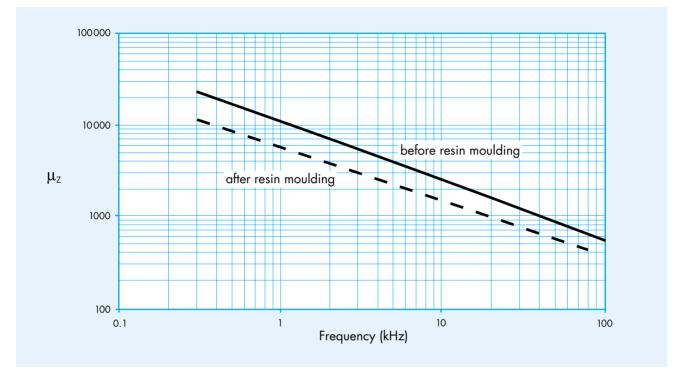
Figure 9 - Typical curves of the impedance permeability μ<sub>z</sub> of Magnifer 8105 So in relation to frequency before and after resin moulding measured using stamped rings of thickness 0.55 mm annealed for 3h at 1050 °C.
