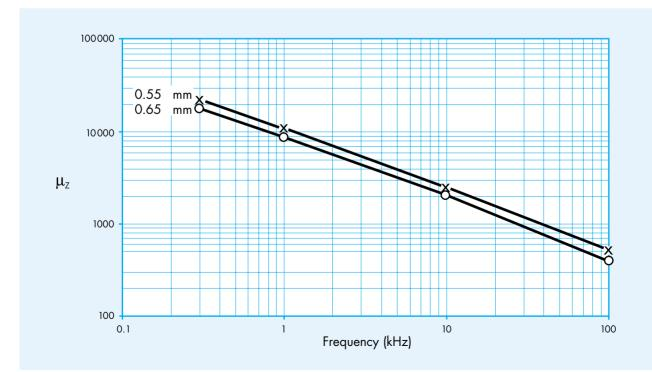
Figure 4 - Typical curves of the impedance permeability  $\mu_z$  of Magnifer 8105 So in relation to frequency and thickness.
