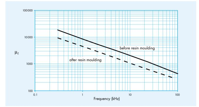
Figure 7 - Typical curves of the impedance permeability μ<sub>z</sub> of Magnifer 8105 in relation to frequency before and after resin moulding measured using stamped rings of thickness 0.55 mm annealed for 3h at 1050 °C.
