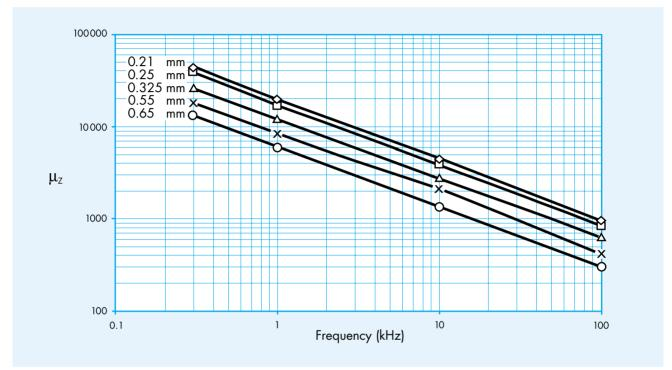
Figure 3 - Typical curves of the impedance permeability  $\mu_z$  of Magnifer 8105 in relation to frequency and thickness.
