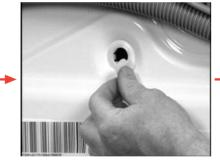
Using the plastic plugs provided, the holes can now be covered.
