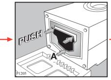
Insert the cover into position. The bottom of the cover «A» should be placed into position first. Not present in all models.
