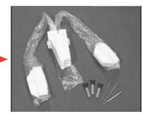
Finally you should have removed from your machine, 3 bolts, 3 spacers and 3 Polystyrene blocks.
