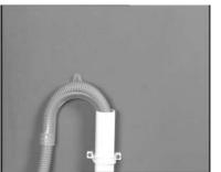
The Drain Hose can be hooked into a standpipe. The hook is formed using the «U» piece provided. The maximum length of hose inside the standpipe must not be more than 30 mm.
