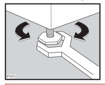
Remember for good stability the machine will need to be level. The feet can be adjusted using a suitable spanner; they incorporate a self-locking nut.
