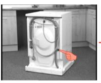
Using a suitable 10 mm spanner remove the right-hand transit bolt only.
