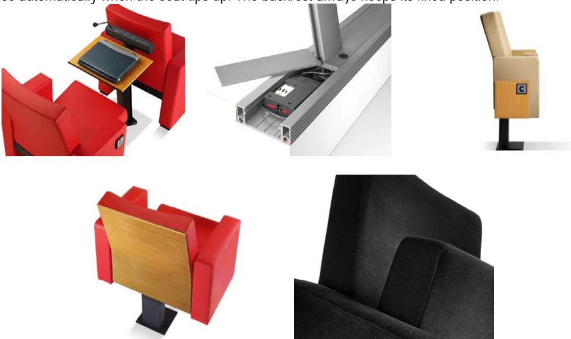
The seat consists of a compact single block of cold moulded polyurethane foam that fully covers the internal metal structure of the seat. This structure comprises a curved tubular frame, a mesh of flat springs and hinge pins for the seat to swivel on. The polyurethane foam block is covered with an easily removable and replaceable zip-on upholstery. The backrest is made in the same manner as the seat.
