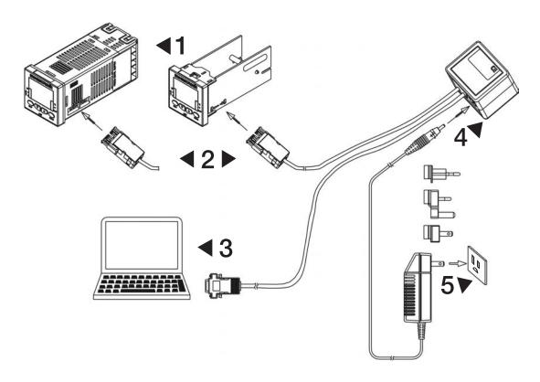
The 1601E can be connected to the remote Configuration Kit, CNFG-10000. This method of configuration is ideal for OEM's for quick setup and for resellers to easily program a controller for the specific needs of a customer.
