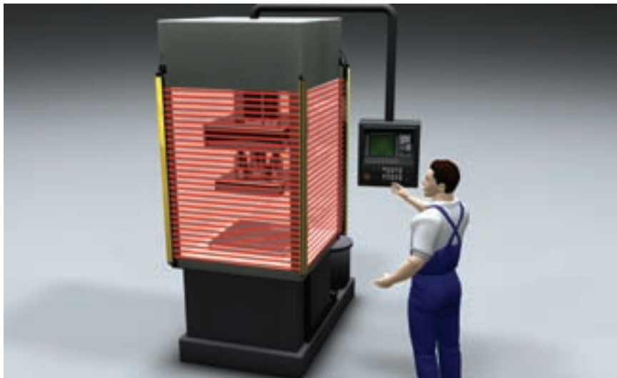
Multiple side point of operation guarding on a press with Safety Light Curtains and beam deflection with Deflecting Mirrors
