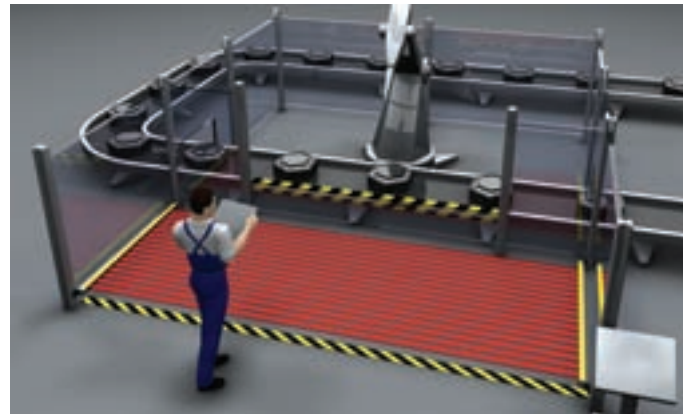
Safety Light Curtain with an MSI Safety Relay, MSI-SR2/F as danger area guarding with start/restart interlock on a robot cell
