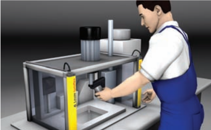
The cycle control function of the MSI safety interfaces allows efficient semi-automatic processes
