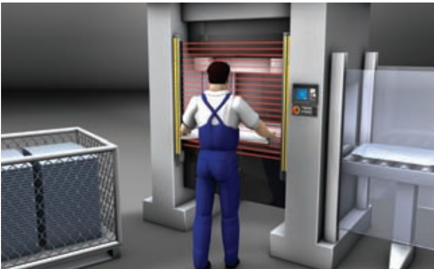
Guarding a compression molding press with automatic unloading and machine initiation using cycle control
