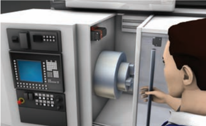
S10 Safety Switch on a CNC rotary machine
