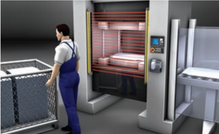
An MSI safety interface with combined cycle control and muting function enables efficient work cycles on a manually fed press
