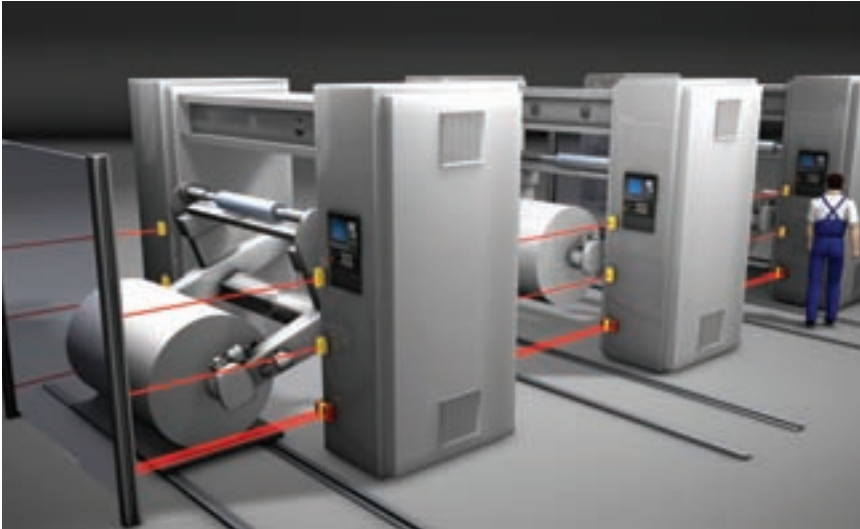
Guarding a printing machine reel changer with SRK 96 single beam safety device
