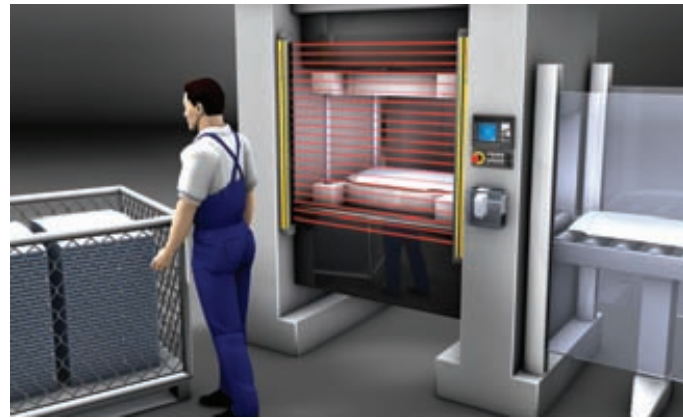
Single-cycle control of an off-centre press with a COMPACT Safety Light Curtain and the MSI-i/R safety interface
