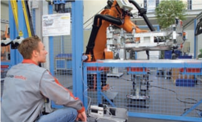
Our stopping time measurements are an important basis for the correct positioning of protective devices
