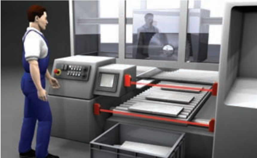
Guarding at a wood processing machine with an SLS 46 Single Light Beam Safety Device
