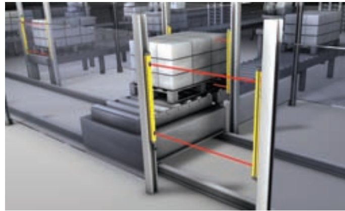
ROBUST guarding with Multiple Light Beam Safety Device on palletizer line
