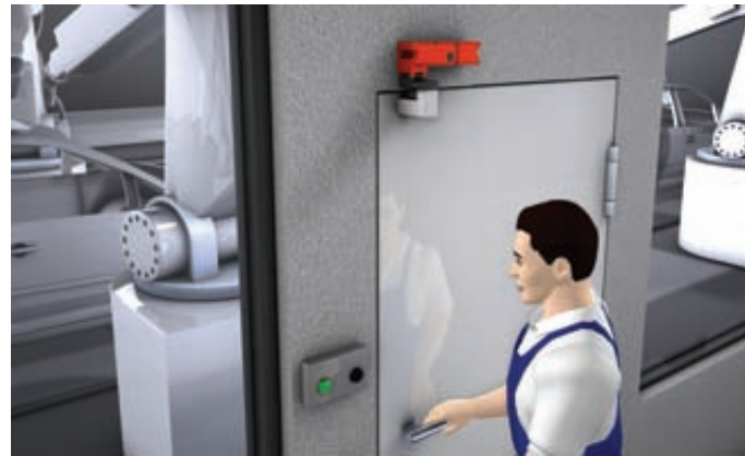
Safety Locking Device as access guarding on an automated system
