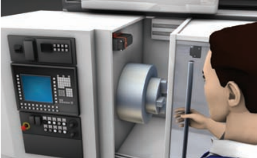
Guarding a CNC rotary machine with S10 Safety Switches and MSI-SR1 Safety Relay
