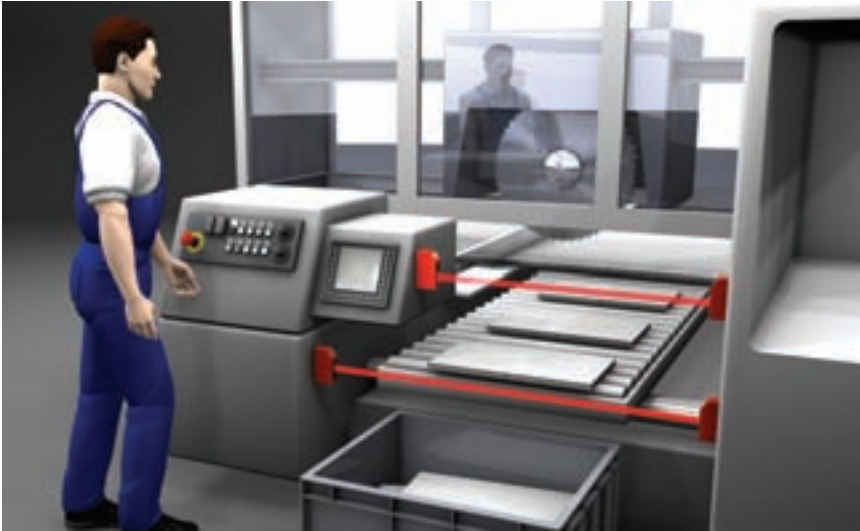
Guarding a wood processing center with SLS 46 Single Light Beam Safety Devices and TNT 35 test monitoring
