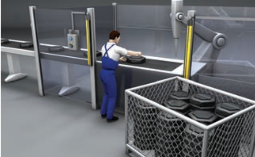
COMPACT plus for point of operation guarding at an automated line
