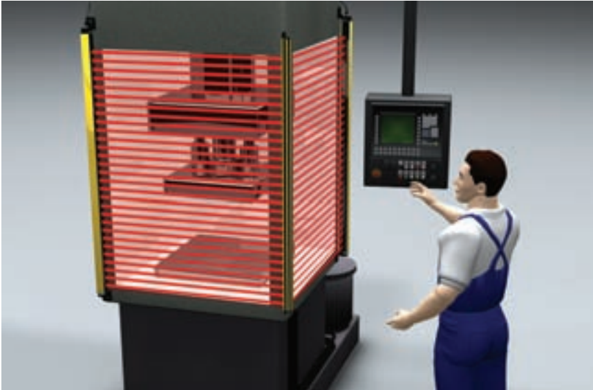
SOLID-4E with 20 mm resolution for hand protection for point of operation guarding on presses
