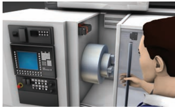
Safety Switches (without guard locking) on a CNC rotary machine
