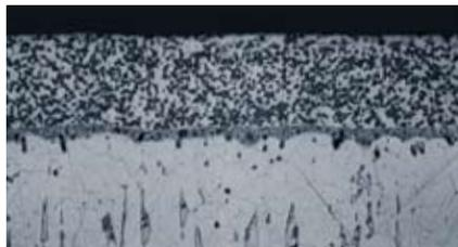
Cross section of EKatex® coating - electroless Nickel diamond dispersion (2 µm)
