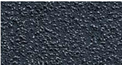
SEM image of EKatex® coating - electroless Nickel diamond dispersion (2 µm)
