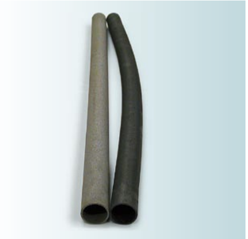
Fig. 2. Kanthal APMT (left) and Fe-35Ni-25Cr (right) after the sagging test.
