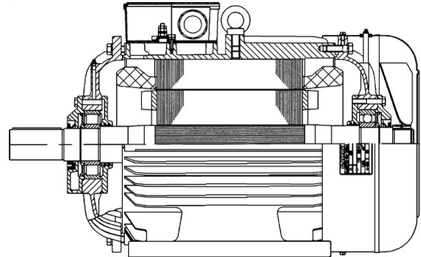
Frame size 280/4-6-8...355 D-End: Roller Bearing
