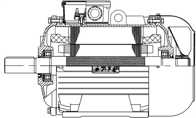
Frame size 63...132 D-End: Floating Ball Bearing (Spring-loaded)
