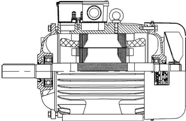
Frame size 160...280/2 D-End: Floating Ball Bearing (Spring-loaded)
