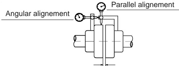
When the motor is coupled to the driven machine, the shafts must be aligned both radially and axially to each other by means of dial gauges. Measurements to be taken at 4 points displaced by 90° each while both coupling halves are turned simultaneously.
