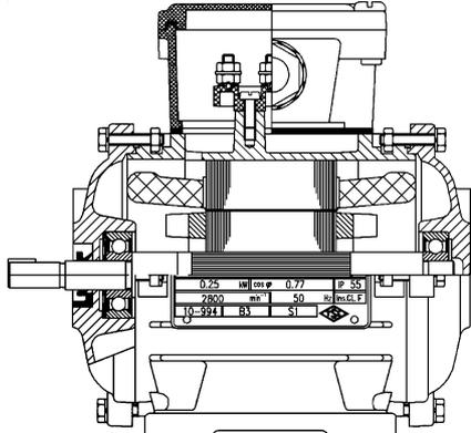
Frame size 56 D-End: Floating Ball Bearing (Spring-loaded)
