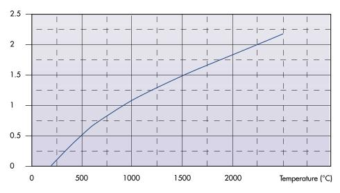
The increase should be added to the typical value of the linear expansion coefficient at 20-200 °C.
