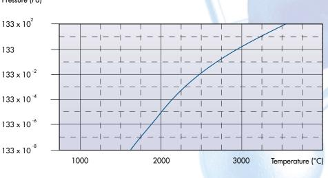
Carbon vapor pressure during high-temperature operation
