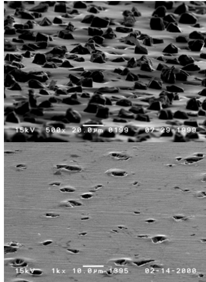
Contact surface of friction joint with EKagrip® friction enhancing shim after assembly and disassembly
