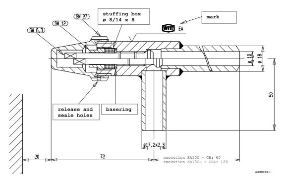
Dimensions for EA 10 G, GL, GBL, GN, G/VA, GL/VA, GB/VA, GN/VA and GNL/VA
