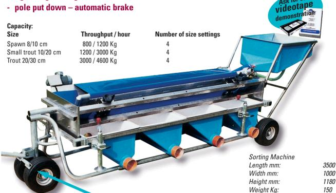
The conveyor belt is driven by a 230/380 V motor. Optionally, a more expensive, 24 V motor is available to power the sorting machine with a truck battery. The undercarriage with pneumatic tyres is made of hot galvanised steel while all other parts are made of stainless steel, plastics and aluminium.
