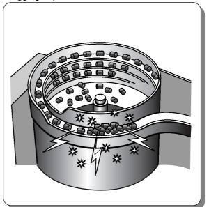
Failures while ejecting workpieces from unloaders
