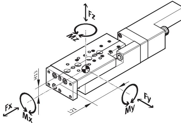
If the drive is subjected to more than two of the indicated forces and torques simultaneously, the following equation must be satisfied in addition to the indicated maximum loads:
