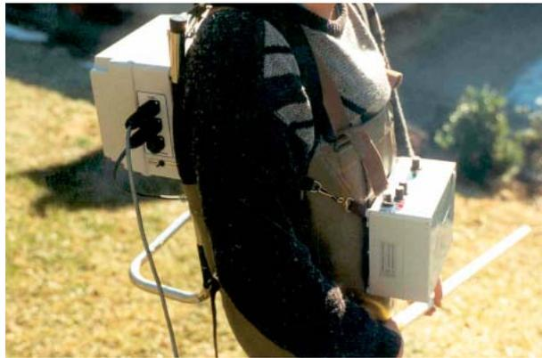
The electronic unit with the controls is attached to the shoulder straps of the battery pack by means of two hooks.
