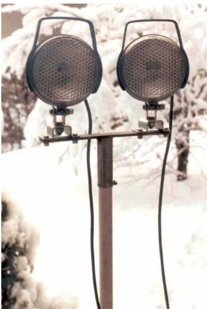
The devices EL65... and EL66... can be equipped with alternators for 110 W power output to power the floodlights. The two halogen lights with 55 W respectively are mounted on the 2 m mast. They can be swivelled and the connecting cable has the suitable connector for the socket of the alternator. The mast slides into a standpipe mounted to the device.
