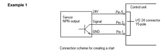
signal by a sensor with NPN output
