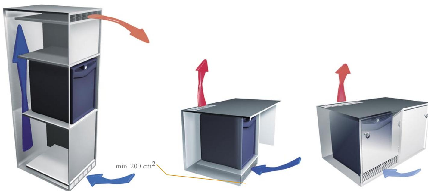
■ Sufficient ventilation can be accomplished even in furniture that reaches higher up. For cooling purposes, the air needs to flow freely around the cooling unit and exit unhindered at the top.
