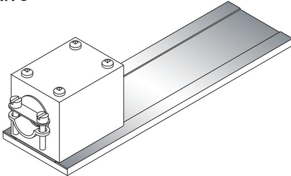
**Sheet Metal Terminal Box-** Available with T2 and T3 threaded terminals.
