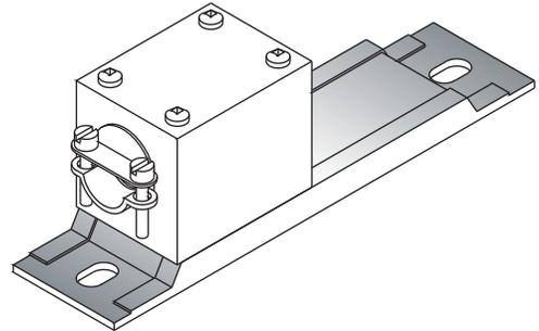
**Sheet Metal Terminal Box-** Available with Type A and C threaded terminals.
