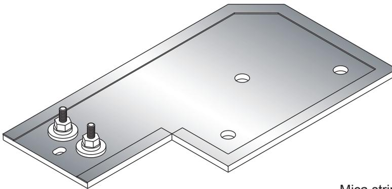
Mica strip heaters are available in irregular shapes and can be made to conform to curved surfaces. Mounting holes aid in clamping the heaters to any surface. Holes and cutouts are useful for the installation of thermocouples and for clearance of bolts and other obstructions
