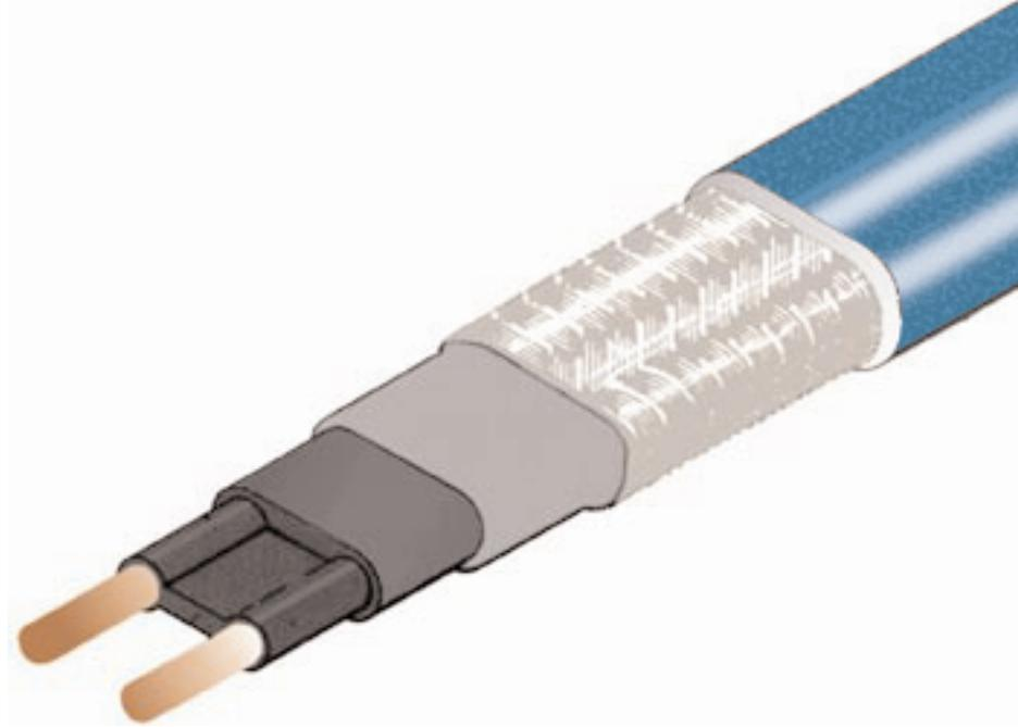
The Devi Pipeheat is a self-limiting parallel heating cable. The power output of the conductive core material increases or decreases in response to ambient temperature changes.
